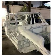
to link the cage to the firewall in the area of the suspension top pivot arm mounts, and this has been done. That improves the articulation between firewall and sills, a known weak point. Less conventional are the pickups for the cage at the rear. The boot structure on a standard car is cantilevered off the sill ends via the D posts, with little or no support from the roof structure or floor pan and the D posts are a weak point.
